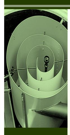
Azar Energy Spiral Separator simulates the natural water power resources for self-cleaning by energetic rotative streams. Oil, sludge and water are simultaneously separated and automatically discharged.
