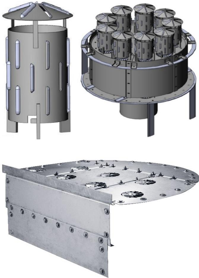
Observational study of flow patterns in centrifugal trays shows that in this kind of trays, gas and liquid passes longer path compared with other trays and it causes increase in residence time, contact area, mass transfer and efficiency.
